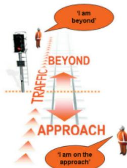
(An example of a signal is given here however it could be a set of points or another fixed structure).
